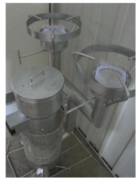
respectively. This difference in start-up time may be attributed to the size of the ignition port, which is smaller for the single-burner stove. Rice husk consumption of the single-burner stove is 1.1 kg per hour while
