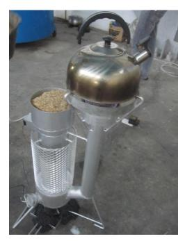
The stove, shown at the right, basically consists of the following parts: a fuel hopper where rice husks are fed; a fan which supplies the air needed for gasification; a reactor where rice husks are gasified using limited amount of air; a gas burner where combustible gases generated are ignited; a gas duct where gas produced is channeled from the reactor to the burner; an ignition port where rice husk fuel is ignited; an adoptor which is used
